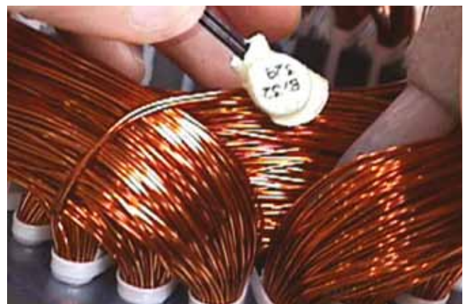
Figure 7.6 - Thermostat installation in the winding
