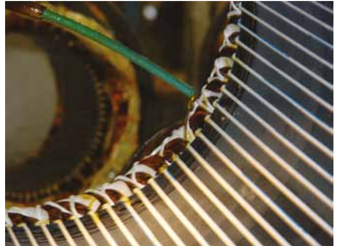
Figure 1.12.c - Resin applied by continuous flow process
